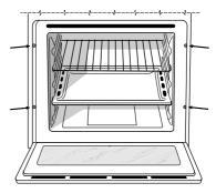
The panels of the adjacent cabinets must be made of heat resistant material. In particular, cabinets with a veneer exterior must be assembled with glues able to withstand temperatures of up to 100°C.
